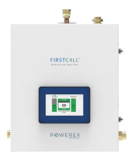
without fluctuation in line delivery pressure. Each bank goes through two stages of pressure regulation, beginning with the dome-loaded bank regulators and then the piston-style final line regulators. After the depleted cylinders are replaced, the manifold automatically designates that bank as the reserve supply, with no manual resetting of valves or levers required.
